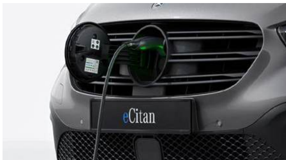
CCS rapid charging port, 75kW max. capacity.
