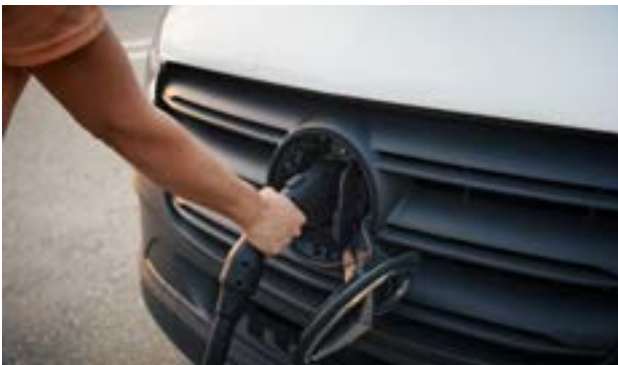
CCS rapid charging port, 115kW max. capacity.
